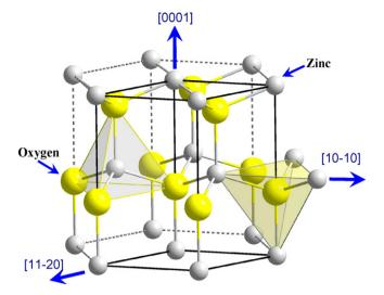
**Fig. 2.** ZnO crystalline structure–Wurtzite structure (modified following Ref. [1]) with directions of  $[0\ 0\ 0\ 1]$ ,  $[1\ 1\ -2\ 0]$  and  $[1\ 0\ -1\ 0]$  indicated. The lattice constants are a=3.25 Å and c=5.2 Å.
