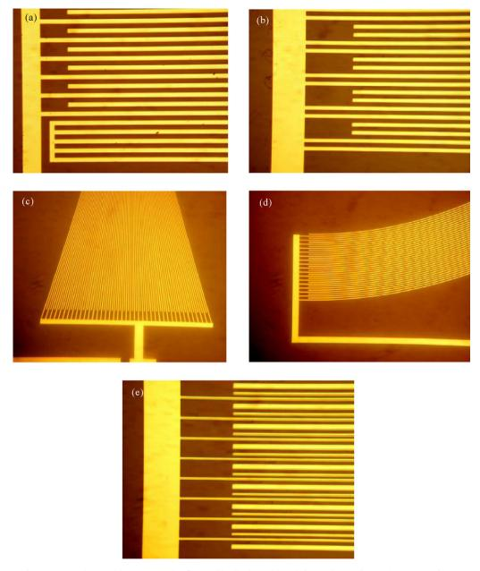
Fig. 7. SAW IDT designs. (a) SAW IDT with reflector; (b) splited IDT; (c) angled IDT; (d) curved IDT; (e) SPUDT IDT design.
