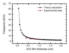
**Fig. 4.** (a) Phase velocities for the Rayleigh and Sezawa modes on different thickness of ZnO film. A film normalized thickness, hk, is used to describe the film thickness effect  $(k = 2\pi/\lambda)$ : wave vector, h: film thickness) [90]; (b) resonant frequency of ZnO FBAR devices vs. film thickness [130].
