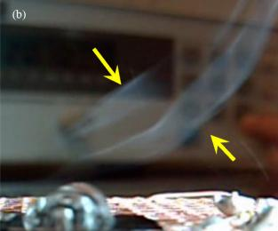
Fig. 8. Surface droplet ejection (a) and atomization process (b) on a ZnO SAW device.
