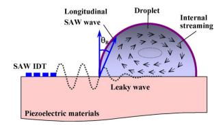
**Fig. 1.** Interaction between propagating surface acoustic wave and a liquid droplet causing acoustic streaming inside droplet.
