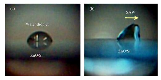
Fig. 6. A 2  $\mu$ l water droplet in (a) and its movement along with the propagating acoustic wave in (b) showing the droplet is pushing upward and forward.
