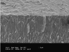
**Fig. 3.** SEM cross-section morphologies of ZnO films deposited using magnetron sputtering method: (a) under target; (b) far away from target showing the inclined structure due to ion channeling effect.
