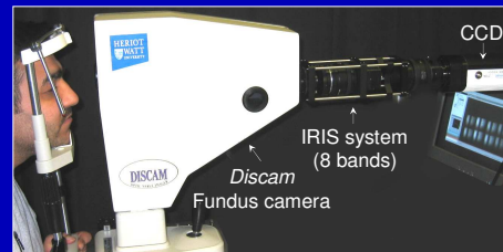
Fig. 2. 8-band IRIS system integrated into Discam retinal camera.
