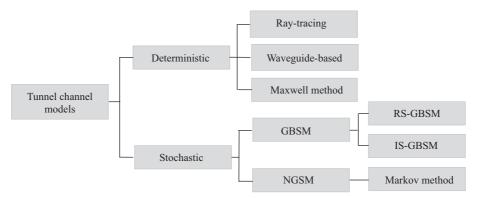
Figure 3 Classification of HST tunnel channel models.
