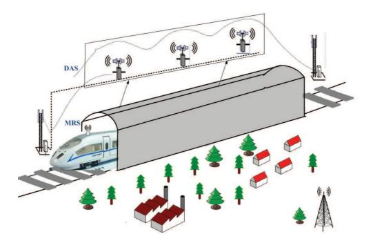
Figure 2 (Color online) HST cellular architecture for tunnel scenario.
