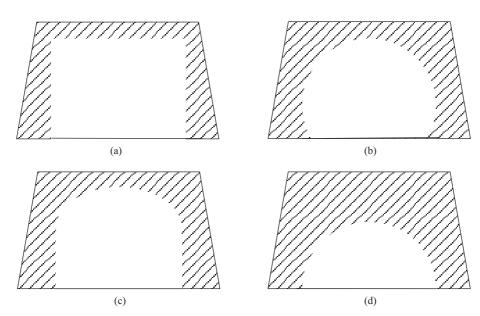
Figure 1 Typical shapes of cross sections for tunnels. (a) Rectangular tunnel; (b) arched tunnel; (c) horse-shoe shaped tunnel; (d) semicircular tunnel.
