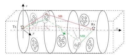
Figure 5 (Color online) A 3D RS-GBSM for HST tunnel scenarios.
